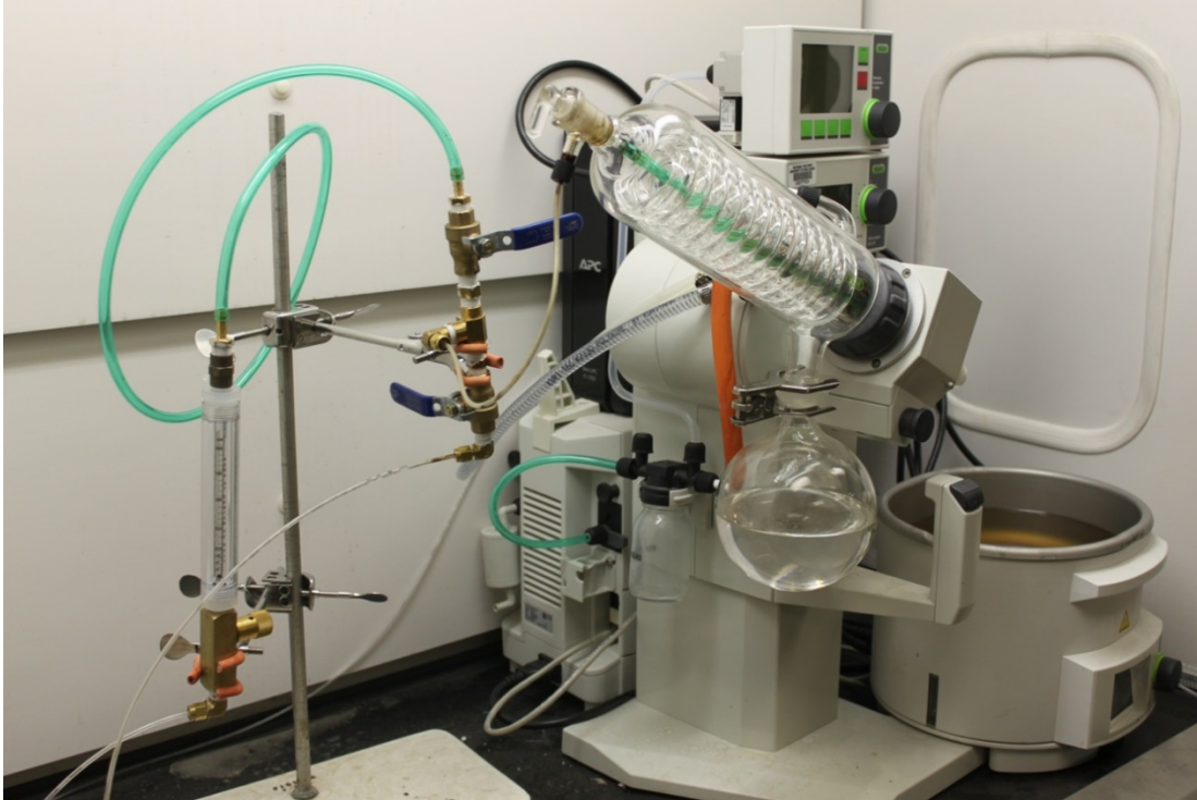
Figure 5 - Asphalt Binder Recovery Equipment at Rutgers University
